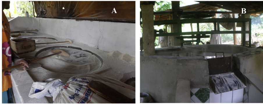
Fig. 4. Roasting systems with a manual furnace (A) and with a motor (B) in Copioba Valley, Bahia, Brazil, 2013.
